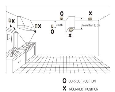
The detector should not be installed:
